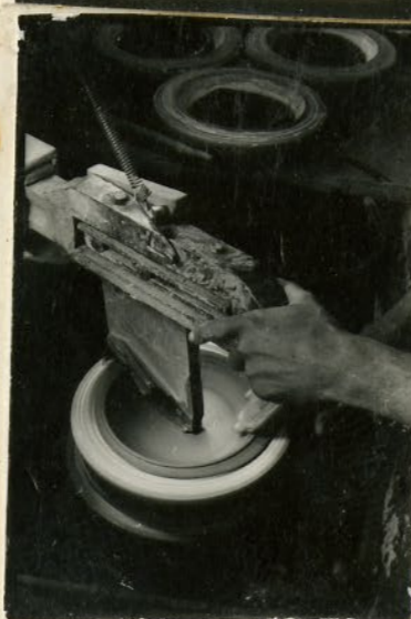
"JIGGERING" MOLDS USED IN PRODUCTION
