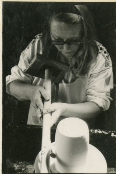
CUTTING MASTER BLOCK FROM WHEEL MOLDS WILL BE MADE
